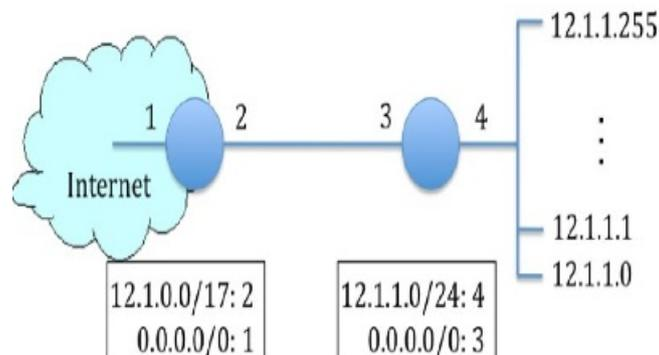
For example, the ISP forwards all packets with destination addresses in 12.1.0.0/17 out link 2 toward the campus edge router. Both routers include a default forwarding entry 0.0.0.0/0 that can match any destination IP address. Answer the following:
